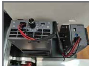
LED Cooling System
